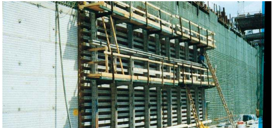
STUDFORM Utilizes aluminum joists and walers to create any size or shape form. Fully adjustable for a wide variety of tie spacings and finishes. Improves workers' productivity, lowers assembly costs and provides for more efficient use of crane time.
